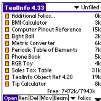
The *Folio List* screen lists the folios installed on the handheld, and allows you to move and manage them.
