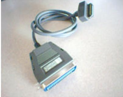
Note that many similar adapters exist for various handhelds and will work. The Greenwich cable is nice in that it's both affordable and runs at 57600 baud. Some other cables are slower, operating at 38400 instead.
